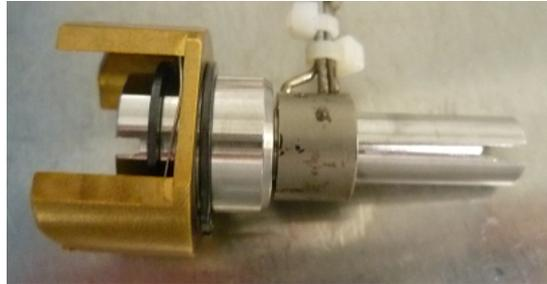
**Fig. 12.** Round heater element mounter
