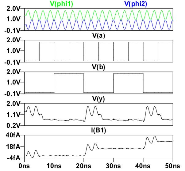
Fig. 5 2PASCL NOR logic circuit with sinusoidal driving voltage.
