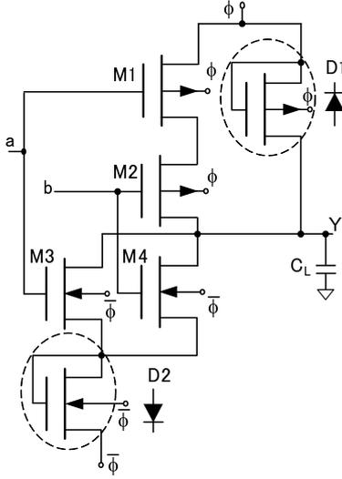
Fig. 3 NOR logic circuit with 2PASCL configuration. nMOS bulk connected to  $\bar{\phi}$  and pMOS bulk to  $\phi$ .
