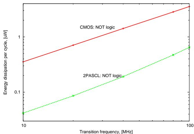
Fig. 1 Energy dissipation of 2PASCL NOT logic circuit compared to CMOS.
