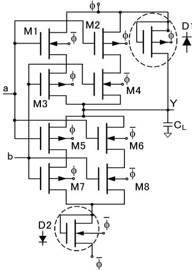
Fig. 4 exclusive-OR logic circuit with 2PASCL configuration. nMOS bulk connected to  $\bar{\phi}$  and pMOS bulk to  $\phi$ .
