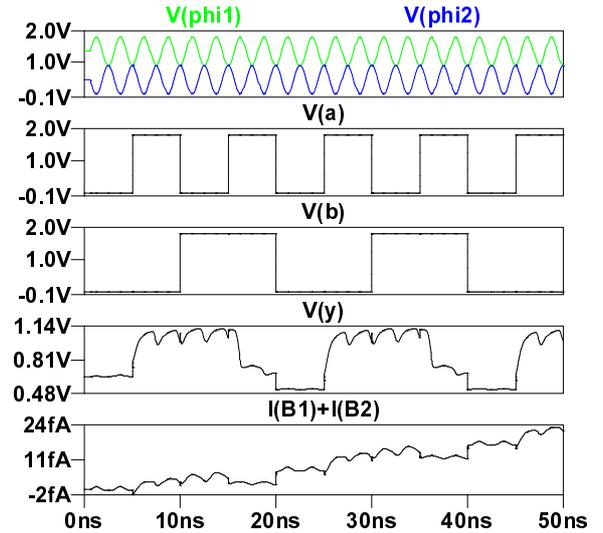
Fig. 6 2PASCL exclusive-OR logic circuit with sinusoidal driving voltage.
