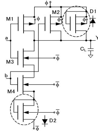
Fig. 2 Leg 2: NAND logic circuit with 2PASCL configuration. nMOS bulk connected to  $\bar{\phi}$  and pMOS bulk to  $\phi$ .
