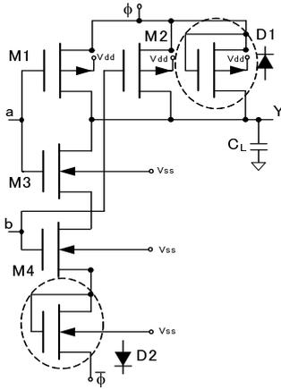
Fig. 3 Leg 3: NAND logic circuit with 2PASCL configuration. nMOS bulk connected to Vss and pMOS bulk to Vdd.
