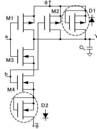
Fig. 1 Leg 1: NAND logic circuit with 2PASCL configuration. nMOS and pMOS connected as existing.
