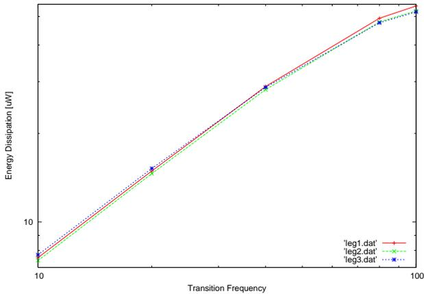
Fig. 4 NAND logic energy dissipation comparison between leg 1,2 and 3.
