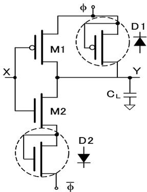
Fig. 1 2PASCL inverter circuit.
