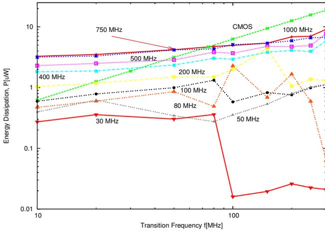
Fig. 3 Power dissipation at different transition frequency.
