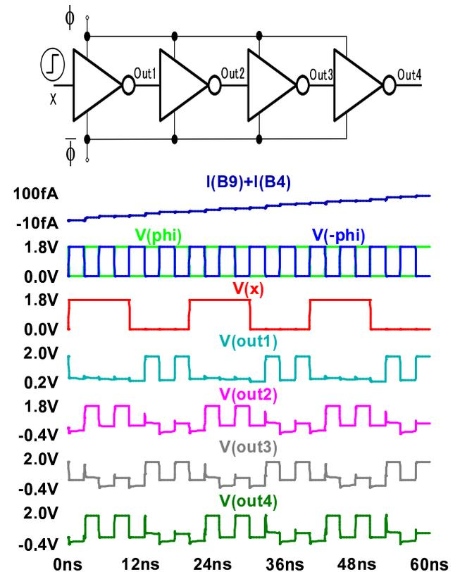
Fig. 2 2PASCL chain inverter circuit and simulation results where clocking voltage is 4 times higher than the input signal.
