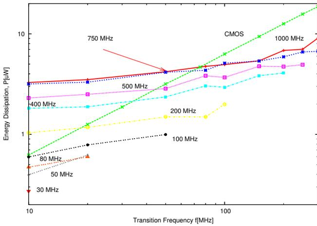
Fig. 4 Power dissipation at different transition frequency minimum clocking signal is 2 times faster than the input signal.
