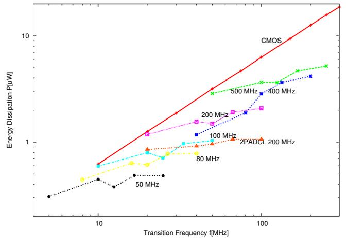
Fig. 6 Power dissipation at different transition frequency where the multiplication of the input frequency is the exact value of the clocking voltage and also comparison to 2PASCL @200 MHz and CMOS.
