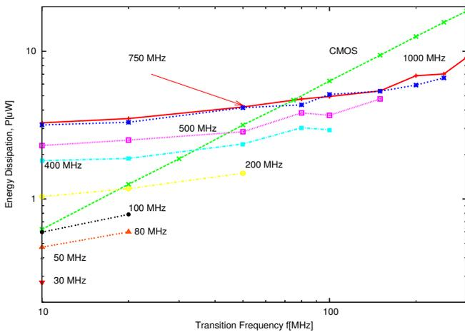
Fig. 5 Power dissipation at different transition frequency where minimum clocking signal is 3 times faster than input signal.
