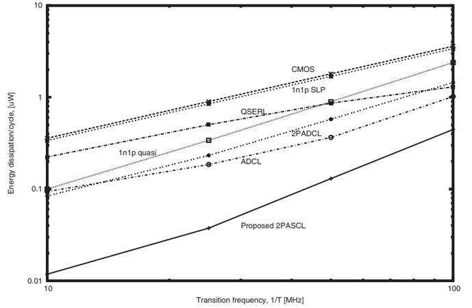
Fig. 8. Energy dissipation comparison for inverter logics.
