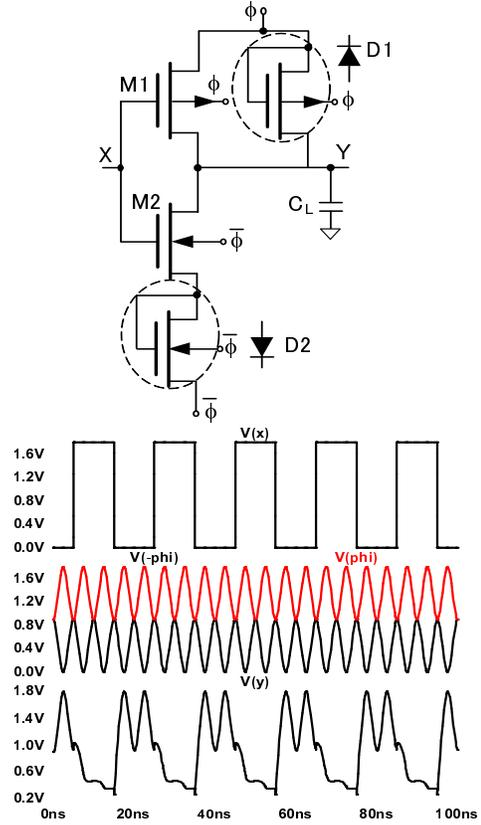
Fig. 1. 2PASCL inverter circuit and its waveforms.
