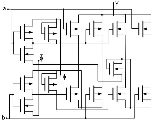
Fig. 3. Schematic for exclusive-OR logic of 2PASCL.
