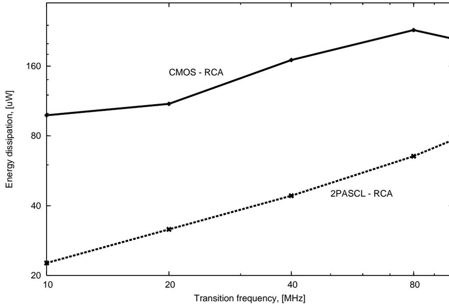
Fig. 6. Energy dissipation comparison with different transition frequency.
