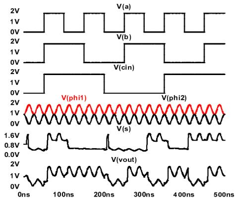
Fig. 5. Output waveforms for ripple carry adder of 2PASCL from the simulation result.
