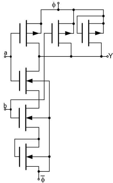
Fig. 4. Schematic for NAND logic of 2PASCL.
