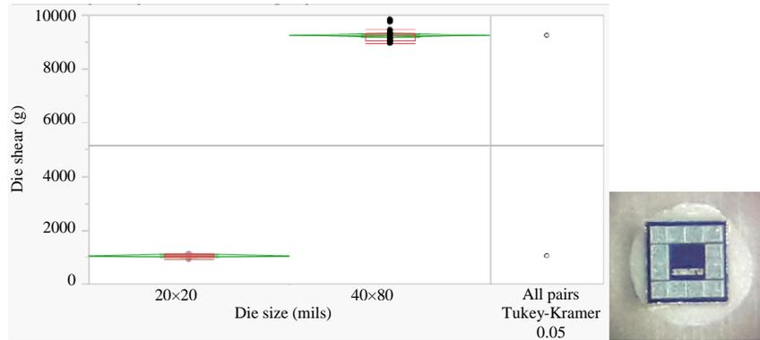
Fig. 8: Die shear test for 20x20 mil vs. 40x80 mil die size (photo)
