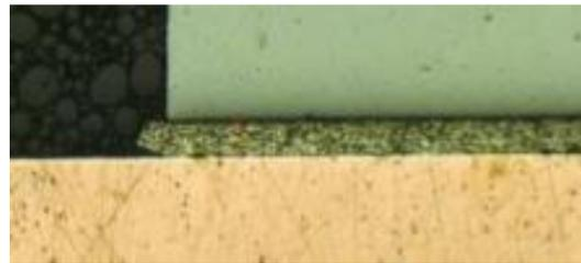
Fig. 10: Two percent void on normal leadframe
