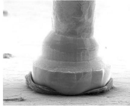
Fig. 13: Bond on high thickness Al bond pad
