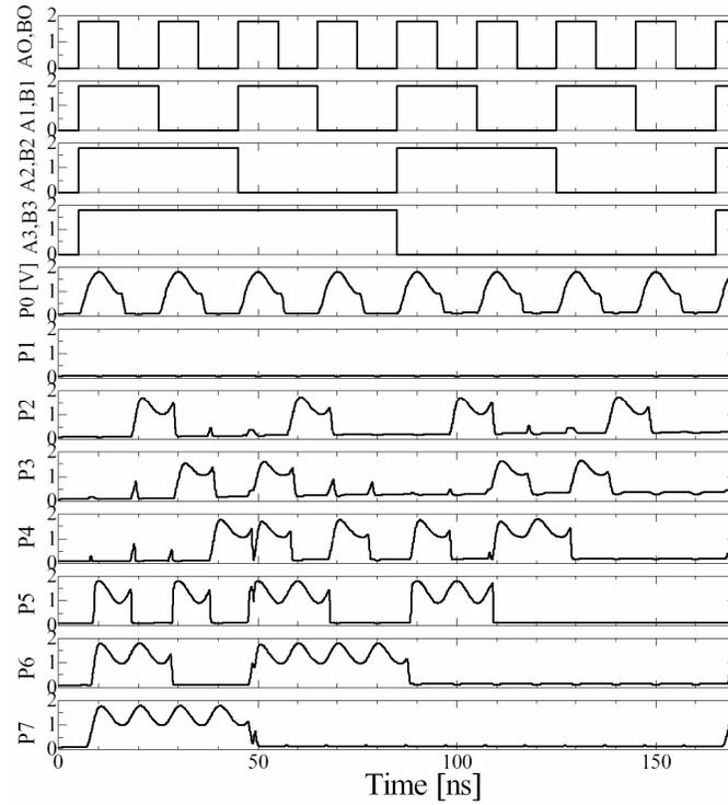
**Figure 8.** Output waveforms of the 4 × 4-bit array 2PASCL multiplier at a transition frequency of 50 MHz obtained from the simulation.
