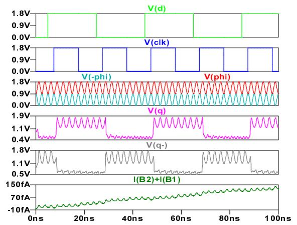
Fig. 6 Simulation output waveforms of clocked D (Data) flip-flop of 2PASCL.
