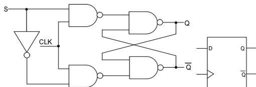
Fig. 2 Clocked D flip-flop.
