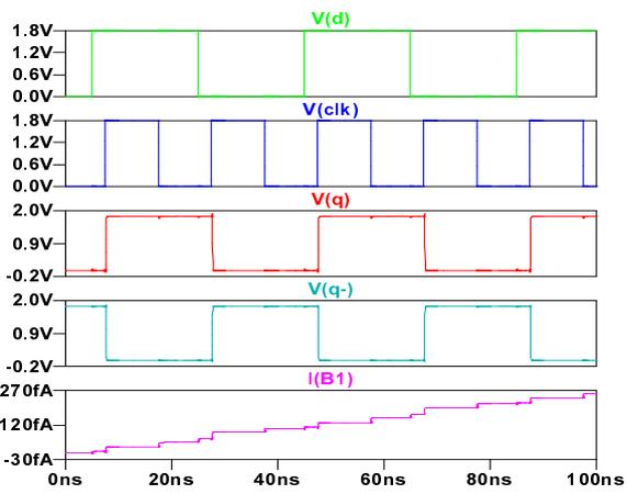
Fig. 5 Simulation output waveforms of clocked D (Data) flip-flop of CMOS.
