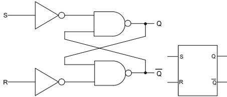
Fig. 1 Set-reset flip-flop.
