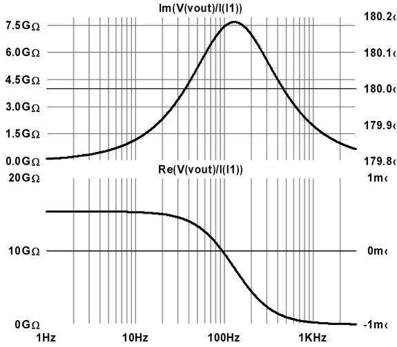
Fig. 5 Bode plot for Hara active inductor.
