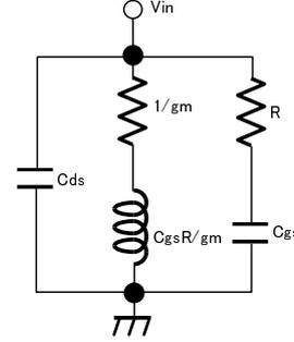
Fig. 3 Simplified Hara active inductor small signal equivalent circuit.
