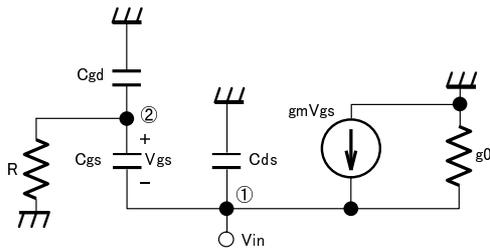
Fig. 2 Small signal equivalent circuit.
