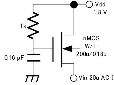
Fig. 6 Hara active inductor with capacitor.
