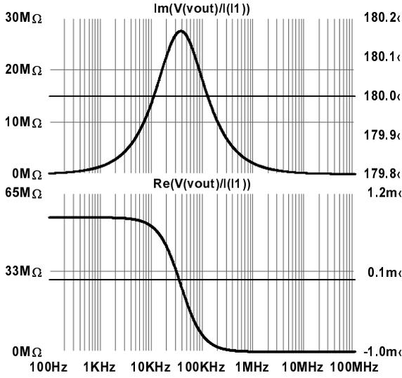
Fig. 9 Hara active inductor with capacitor Bode plot.
