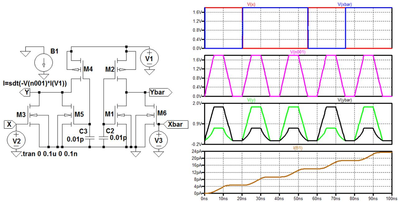
Fig. 5 2n-2n2p quasi-adiabatic logic inverter circuits diagram and waveforms
