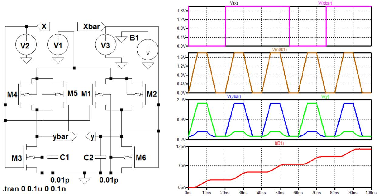
Fig. 1 2n2p-2n adiabatic logic inverter circuits diagram and waveforms
