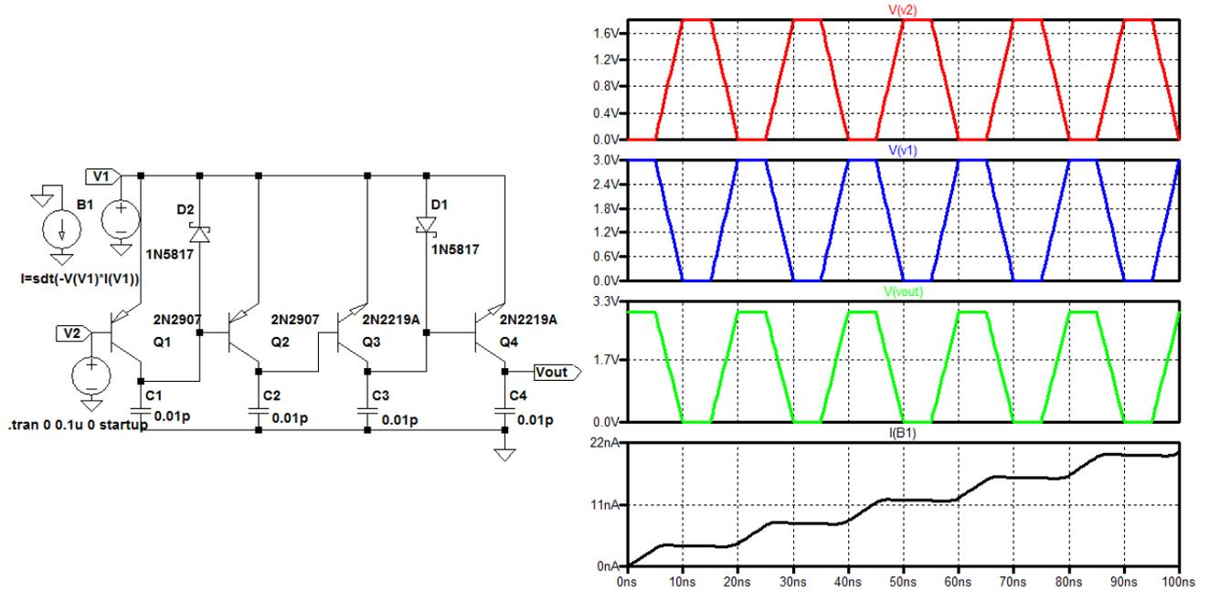
Fig. 7 Recovered-energy logic (REL) inverter circuits diagram and waveforms
