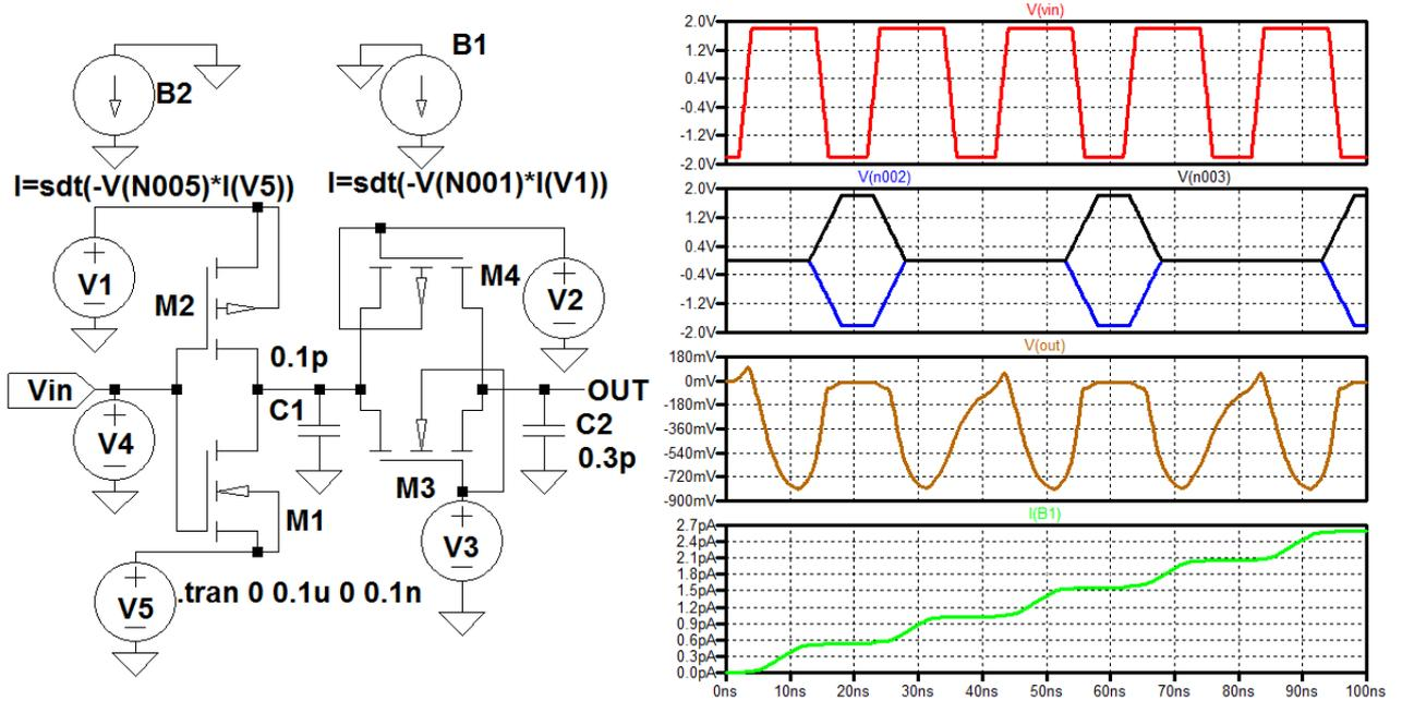
Fig. 3 Split level charge-recovery logic inverter circuits diagram and waveforms
