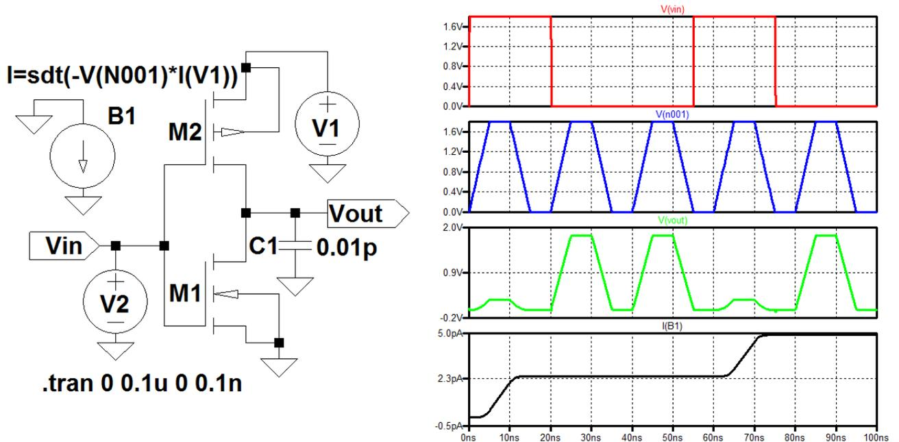
Fig. 4 1n-1p quasi-adiabatic logic inverter circuits diagram and waveforms
