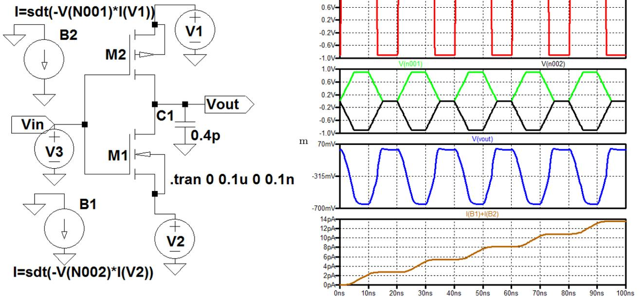
Fig. 2 Split level pulse 1n1p logic inverter circuits diagram and waveforms
