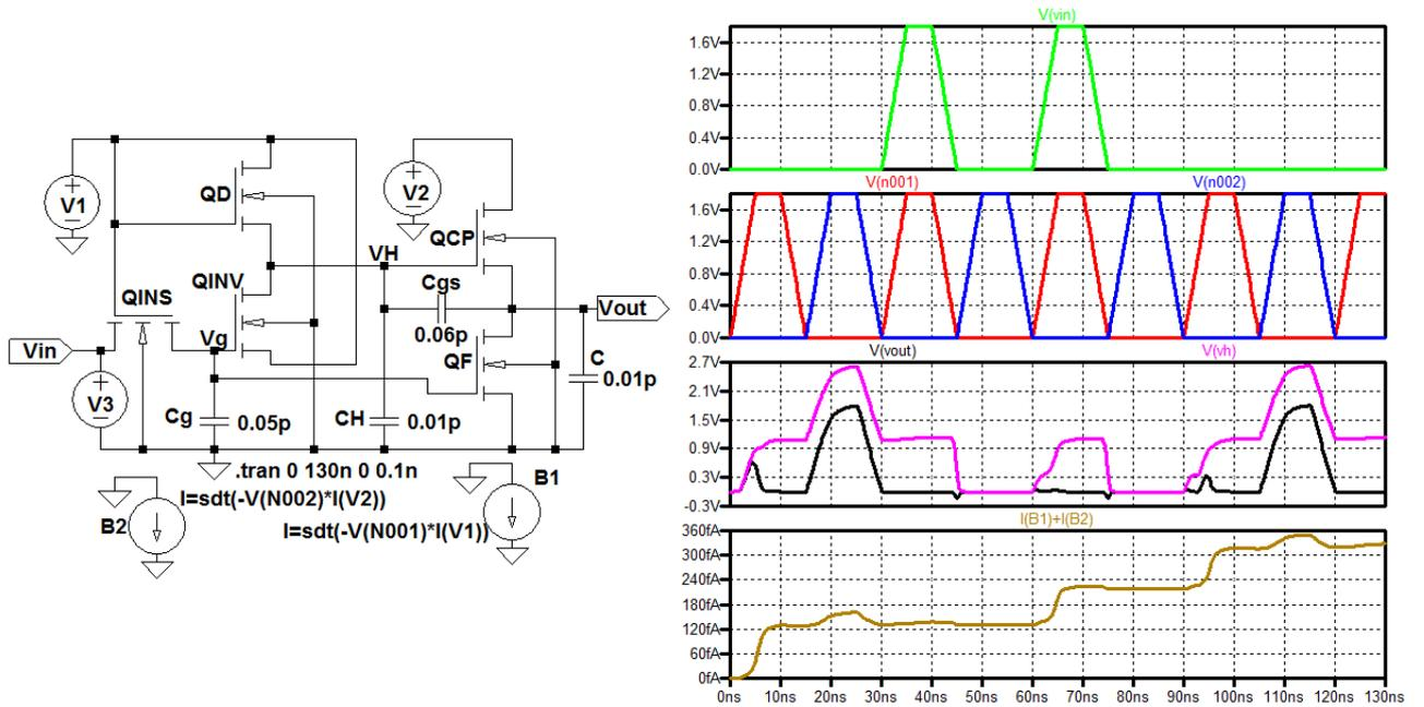
Fig. 6 Hot-clock nMOS logic inverter circuits diagram and waveforms
