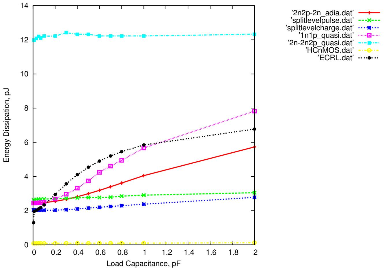
Fig. 11 Energy dissipation comparison in adiabatic circuits at different load capacitance value
