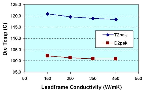
Fig. 6 Highest temperature for T2PAK and D2PAK
