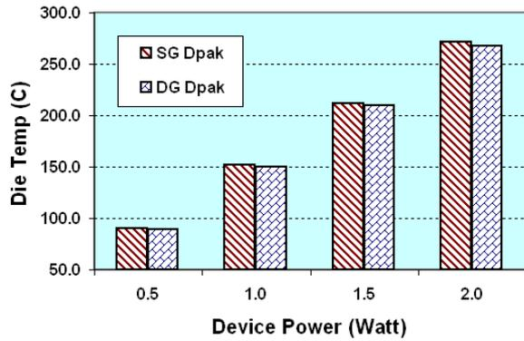
**Fig. 10 Highest temperature for SG DPAK & DG DPAK**
