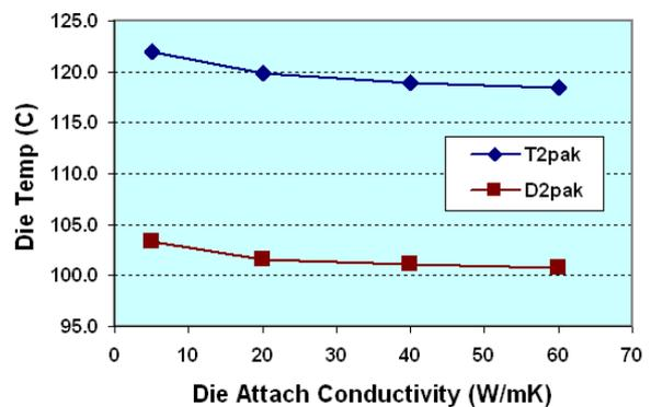
Fig. 8 Highest temperature for T2PAK and D2PAK
