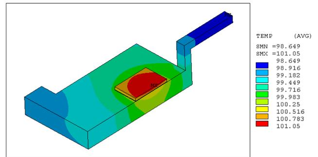
Fig. 7 Temperature distribution of D2PAK
