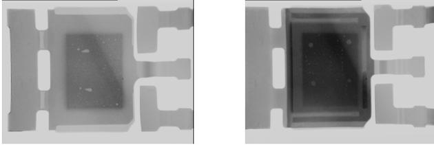
**Fig. 14 No significant die attach void for SG DPAK (left) compared to DG DPAK (right)**
