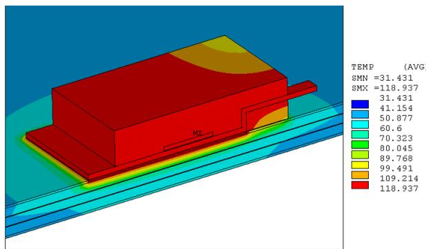
Fig. 5 Temperature distribution of T2PAK
