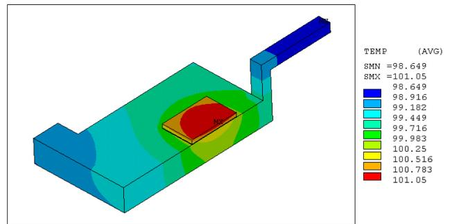
Fig. 7 Temperature distribution of D2PAK
