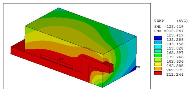
Fig. 9 Temperature distribution of SG DPAK
