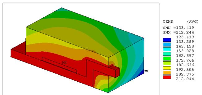
Fig. 9 Temperature distribution of SG DPAK
