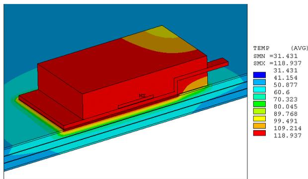
Fig. 5 Temperature distribution of T2PAK
