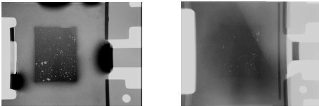
**Fig. 15 No significant die attach void for T2PAK (left) compared to D2PAK (right)**
