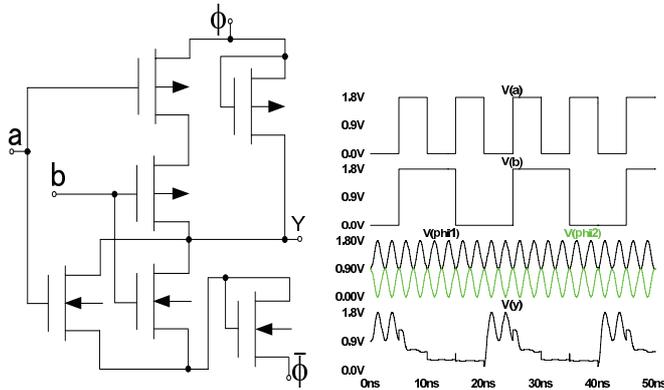
Fig. 10. Scheme for 2PASCL based NOR logic (left), waveforms from the simulation where the output  $Y = a + b$  (right).
