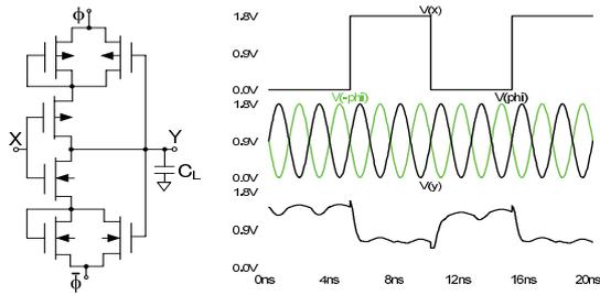
Fig. 5. QSERL inverter and waveforms from the simulation.
