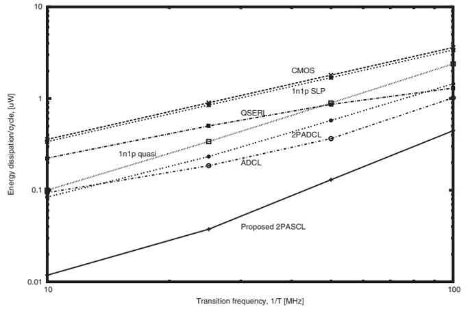
Fig. 8. Energy dissipation comparison for inverter logics.
