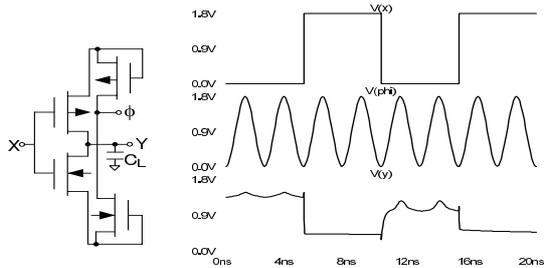
Fig. 6. ADCL inverter and waveforms from the simulation.
