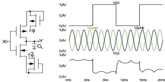
Fig. 7. 2PADCL inverter and waveforms from the simulation.
