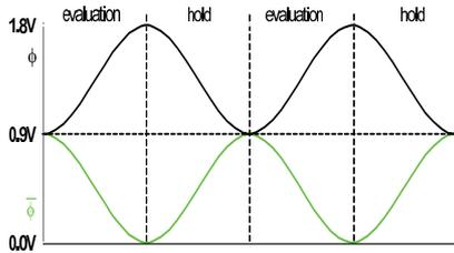
Fig. 2. Clocked voltage driver showing the *evaluation* and *hold* phase.
