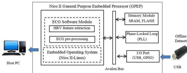
Figure 1: ECG-SoC Cyclone II FPGA.
