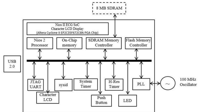
Figure 2: ECG-SoC hardware system configuration
