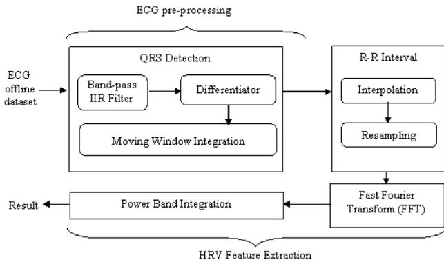
**Figure 3:** Block diagram of ECG pre-processing and HRV feature extraction
