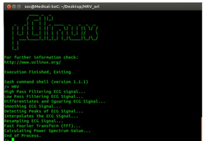
**Figure 4:** ECG-SoC execution in uCLinux
