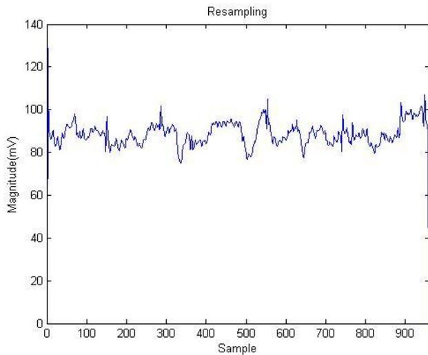
**Figure 9:** Resampling at 4 Hz by employing linear interpolation
