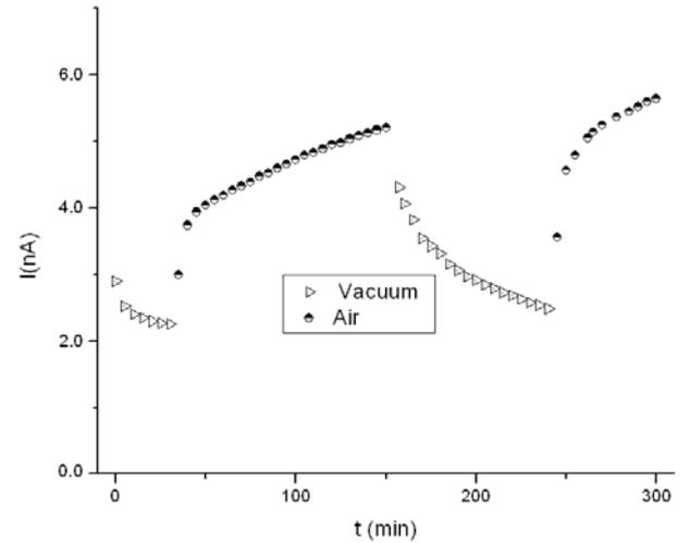
**Fig. 4** Effects of exposing air on the photoconductivity.
