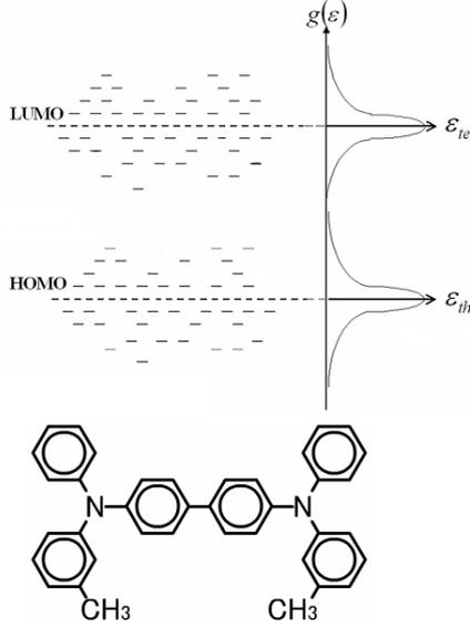
**Fig. 5** Expected energy diagram for disordered TPD films, together with the structural unit.
