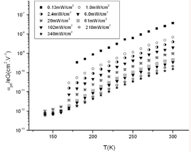
**Fig. 3** Temperature variation of normalized photoconductivity,  $\sigma_p/eG$  ( $= \eta\mu\tau$ ) as a function of  $G$
