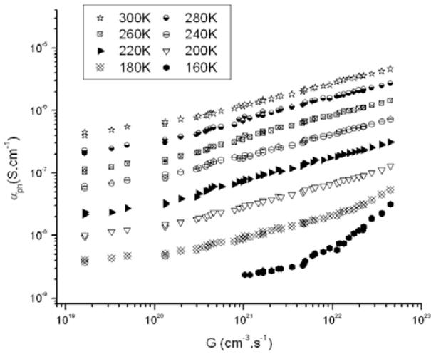
**Fig. 2**  $G$ -dependent photoconductivity of the TPD films as a function of temperature
