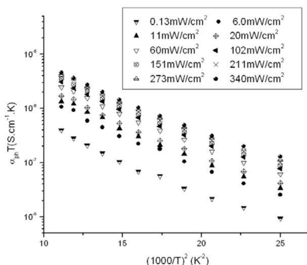
**Fig. 1** Temperature variation of photoconductivity of TPD films, plotted as  $\sigma_{\text{ph}}T$  vs.  $(1000/T)^2$ , as a function of light intensity.
